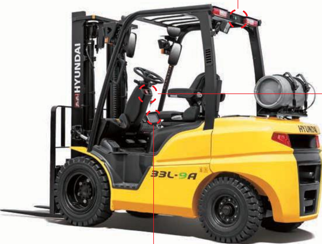
Parking Brake Switch With auto parking function when the operator is not in the seat
