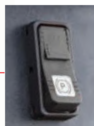
Parking Brake Switch With auto parking function when the operator is not in the seat
