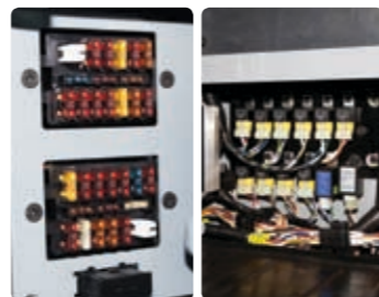
Compact fuse box for easy inspection
