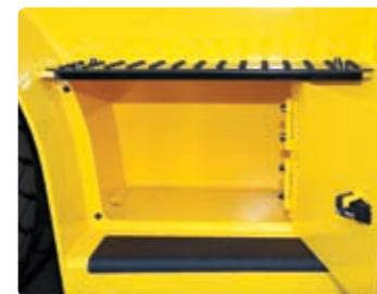
Large tool box Additional tool box located in machine side for operator's convenience.
