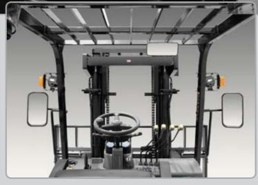
New high visibility for safe operation The operator is able to work with increased safety and accuracy due to a wider view mast
