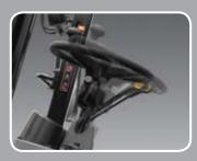
Adjustable steering wheel Steering wheel with horn button can be adjusted by a lever on the right-hand side for the most comfortable operator position.
