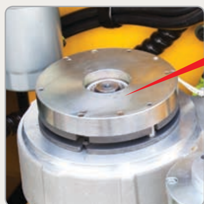
Electromagnetic brake is mounted on the traction motor.
