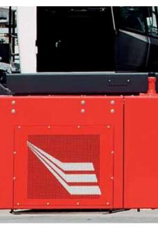
he manually sliding cab leaves complete access to the engine and transmission bay and routine maintenance tasks are made easier by conveniently repositioned fluid level refill cum check points and filters. The roomy Electric System compartment contains and protects the already all-weather proof IP 67 main electric box and system components.
