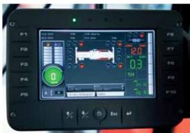
he CVS FERRARI RSE Empty Container Handling Reach Stacker is coming with the supreme comfort and standard options rich CVS FERRARI ARIA cabin, that is air pressurized, excellently sound proofed and fitted with sun glare reflective glasses. The state-of-the-art joystick is capacitive type and the on-board computer has a large, graphic and colour display.
