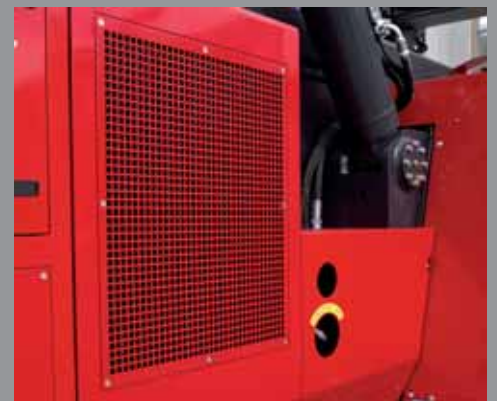
Oversized Hydraulic Oil cooling
