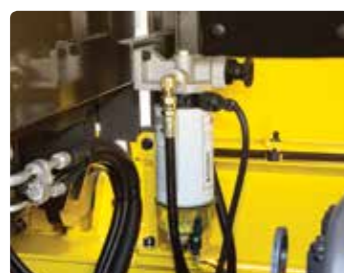
Mechanic Friendly Fuel Filter Replacement
