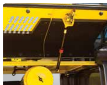
Automatic Self Locking Gas Spring
